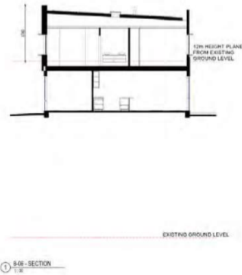
Figure 14. Proposed dwelling 8-06 section depicting existing ground level and 12m height overlay (red dashed lines)
