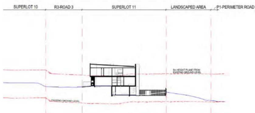
Figure 55: Extended long section through Lot 11.01 showing the transition from the existing Perimeter Road to the south through to superlot 10 which, previously discussed, is serviced by, and thus fixed to, the existing retained Perimeter Road to the west (source: Mirvac Design)
