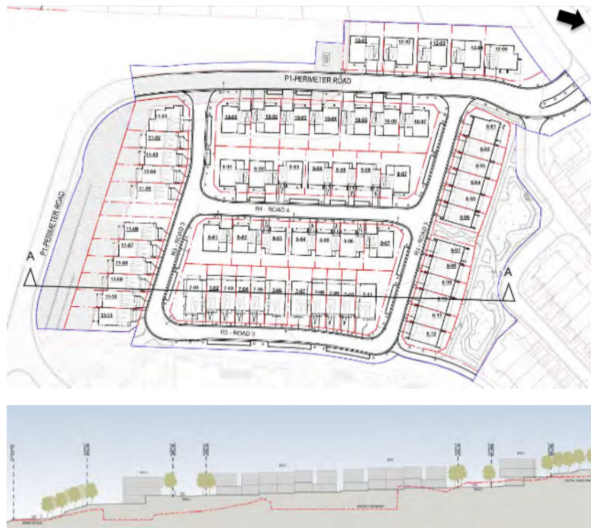
Figure 12: Plan with lot numbers and Section A-A taken through superlots 6, 9 and 11 highlighting the transition of existing topography and proposed finished ground level of the site. (Source: Mirvac Design)
