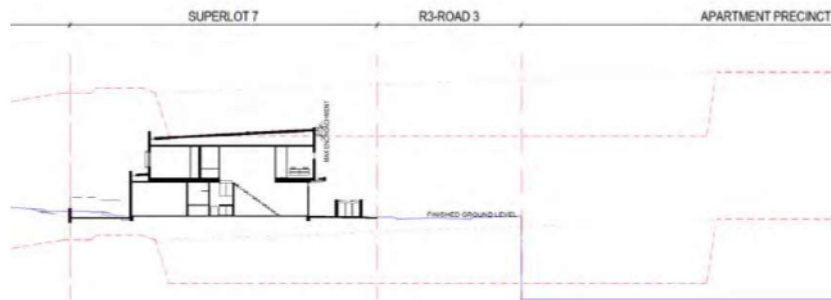
Figure 17: Extended section of 7-03 depicting extrapolated ground level across existing building basement location (grey dashed line. Source: Mirvac Design)
